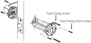
To attach privacy furniture to the door fit the threaded spindles to one side of the backplate first then insert the square spindle. Then offer up to the door and fit the thumb turn furniture. Screw the machine screws into the spindles. Then add extra wood screws for strength.
